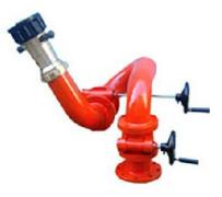
Stand post monitors are used in fire fighting for applying large quantity of water/foam from a distance onto the risk area. The monitors are normally installed onto stand posts, fitted onto the fire water network, or mounted on trailers/trolleys. Geared swivel joints allow operator to effortless change/adjust the position of the monitor using hand wheels, if required.
